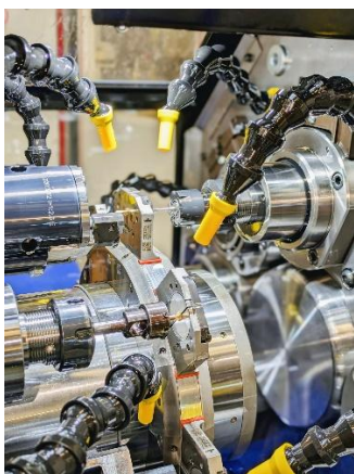
Image 11: The indexing table advances workpieces from one station to the next, where stationary, non-rotating parts are machined simultaneously by powered tools.
