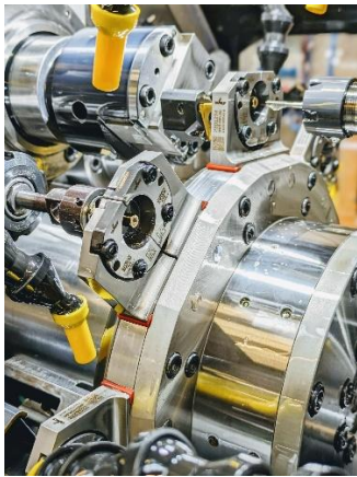
Image 10: At the heart of the Wolf TSM 280 is a vertically arranged clamping table with eight or sixteen hydraulically actuated workpiece holders.
