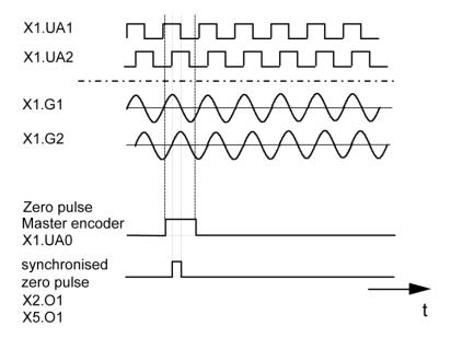
Sine wave encoder signals (only from I type encoder) or square wave signals can be fed through input X1 of the AP-IF3 module.
