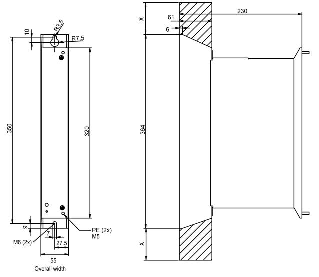
X free space for convection cooling distance both sides min. 60
