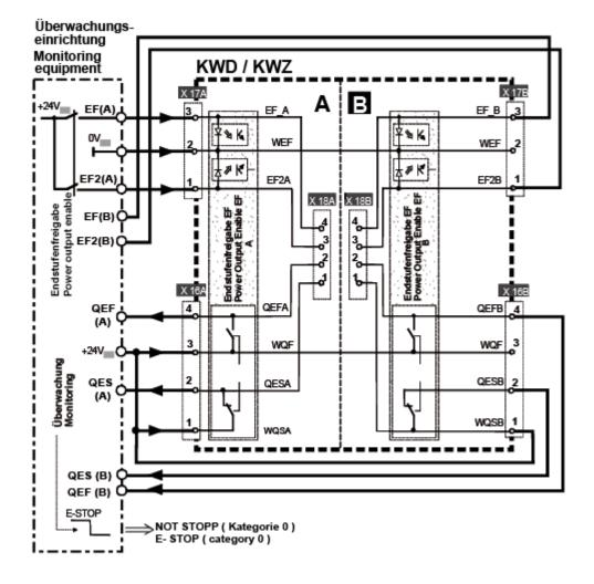
Power output enable single safety (A/B), two-channel (EF and EF2):
