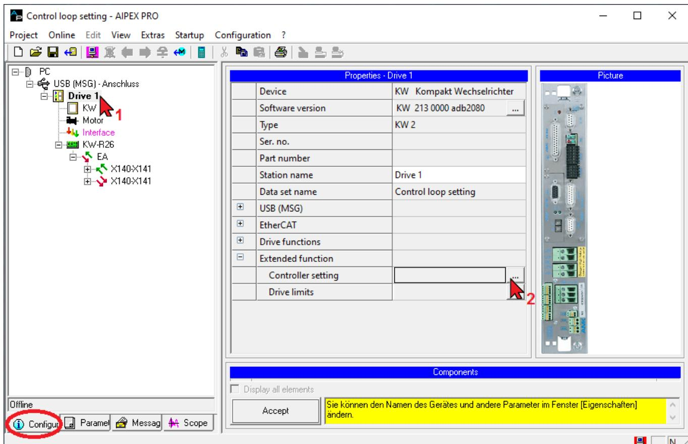
You will find the control setting under 'Extended function', in the 'Configuration' tab and the 'Properties' window.
