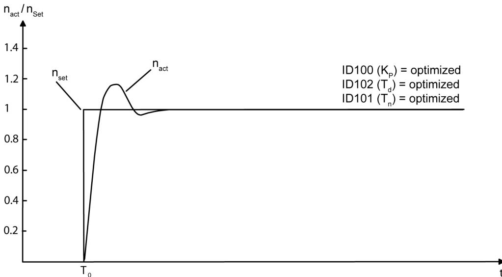
For an optimally set PID controller, the actual speed value may overshoot a setpoint step-change by no more than 20%.
