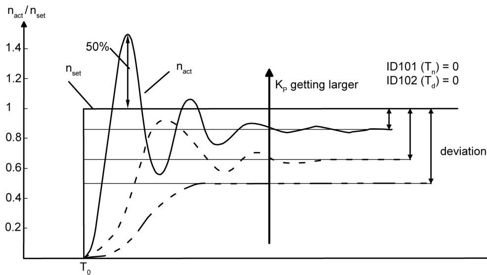
Halve the determined value for 'Speed control proportional gain KP'  $K_p$  and enter the halved value in ID100.
