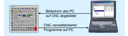
The display of the CNC is illustrated on a PC. The control can be served then from the PC.
