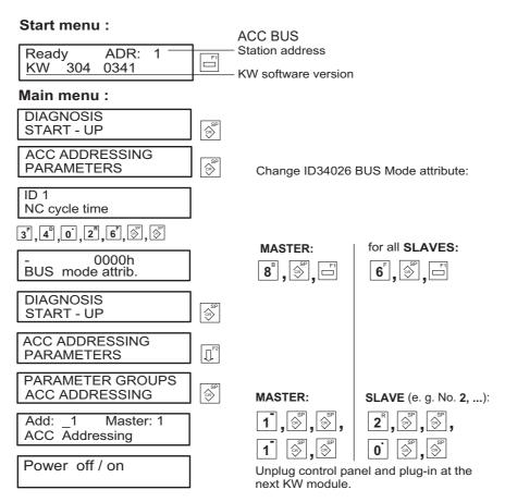
After parameter setting on all KW modules: POWER (24V supply voltage) OFF and ON again after approx.10s.
