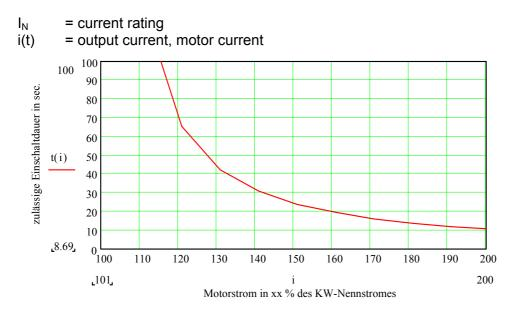
Motorstrom in xx% des KW-Nennstromes = Motor current in xx% of the KW current rating zulässige Einschaltdauer in sec. = Permitted on-time in sec.
