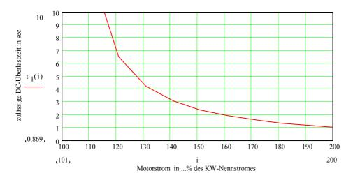
Motorstrom in  $\dots$ % des KW-Nennstromes = Motor current in xx% of the KW current rating zulässige DC-Überlastzeit in sec. = Permitted CD overload time in sec.
