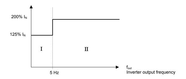
For the **operation range** I with inverter output frequencies of less than 5 Hz a maximum motor output current of 125 % of the nominal current of the KW device is permitted.
