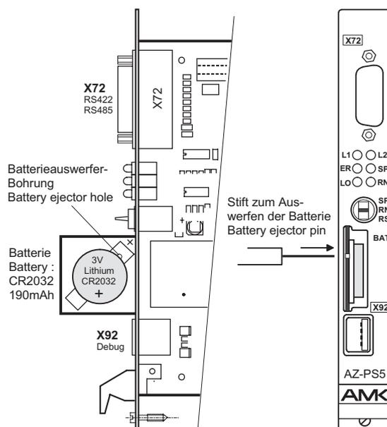
**AZ-PS5 Serial interface: RS422 (RS485 capable)**
