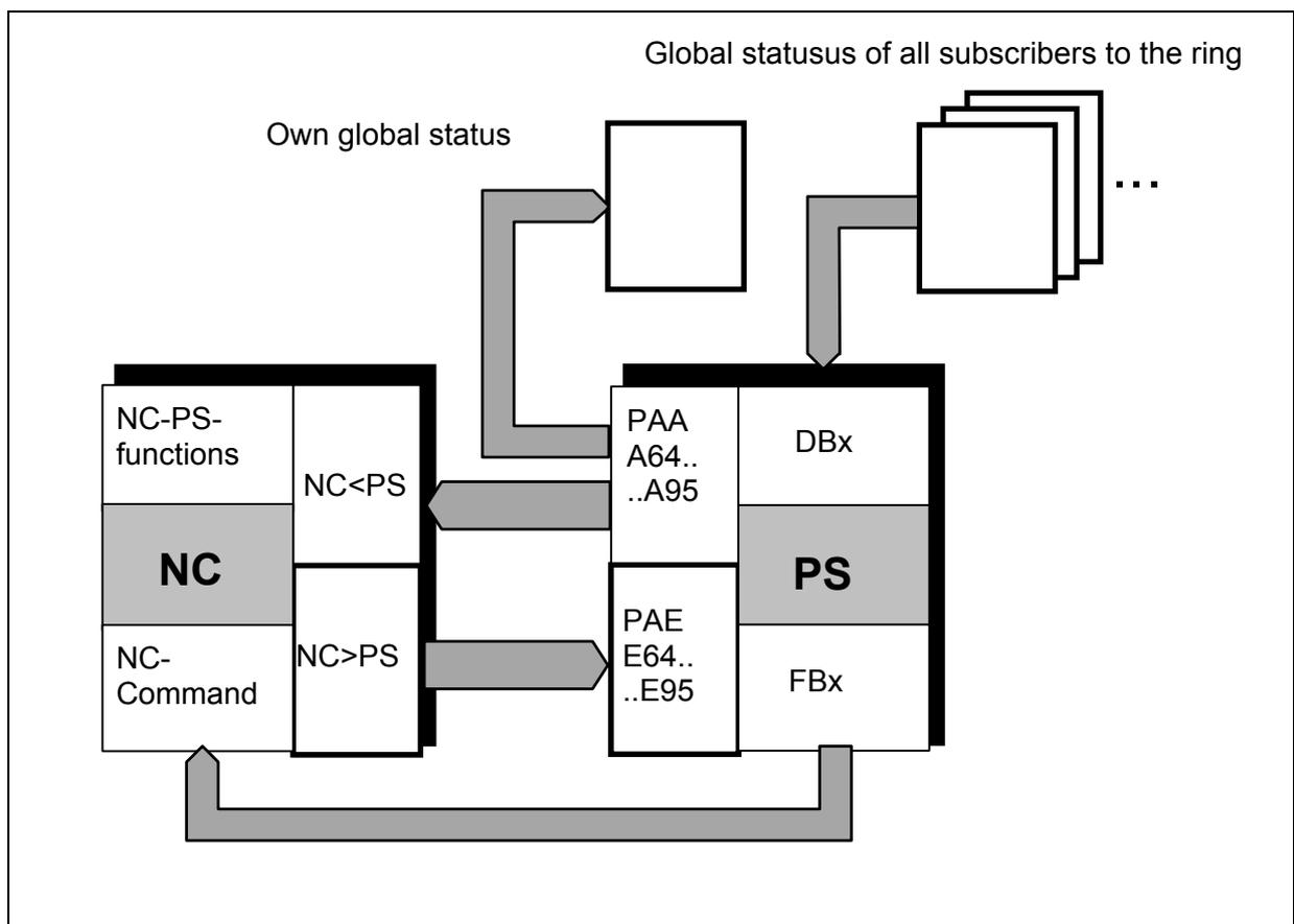
Fig.1: Block schematic of NC-PS interface (shown here for channel 1)
