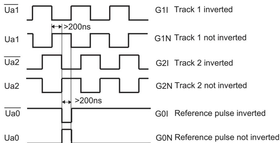
The maximum input frequency is 1 MHz, **from Rev. 1.05: 500kHz !**
