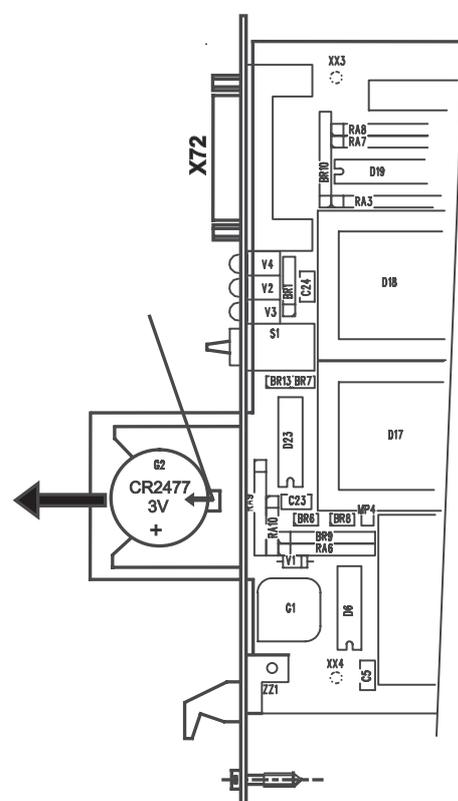
**AZ-RC1 component mounting diagram and front panel**
